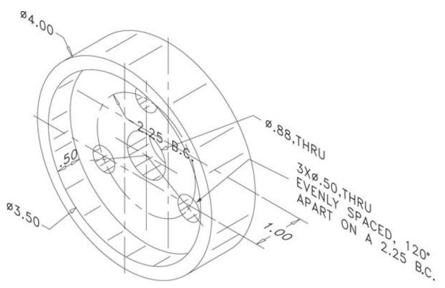
(B.C. stands for bounding circle. In other words, the centers of the holes lie at the same radial distance from the center of the bounding circle, which is also the center of the part.)
