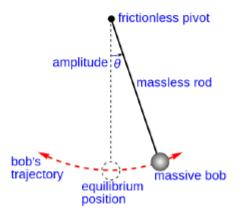
Assume that the length of the rod is L and the mass of the bob is M. the angle of the pendulum with the vertical axis is denoted by  $\theta$  and is shown in the figure. (The direction of the arrow denotes the positive direction for  $\theta$ .) Assume that there is a motor at the pivot point which applies torque T to the pendulum. Assume that the pendulum is oriented up and operates close to the second equilibrium point.
