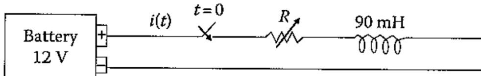
(a) Calculate and plot the battery discharge current,  $i(t)$ , if the steady-state discharge rate is  $C/3$  in Ah/h (C is battery rated capacity). Neglect battery voltage drop.
