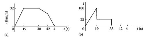
Calculate the EV range based on SAE J227a schedule B driving cycle using the power density approach of fractional depletion model (FDM). You assume that there is no regenerative braking. The drive cycle and current profile of the EV is shown in the above figure.
