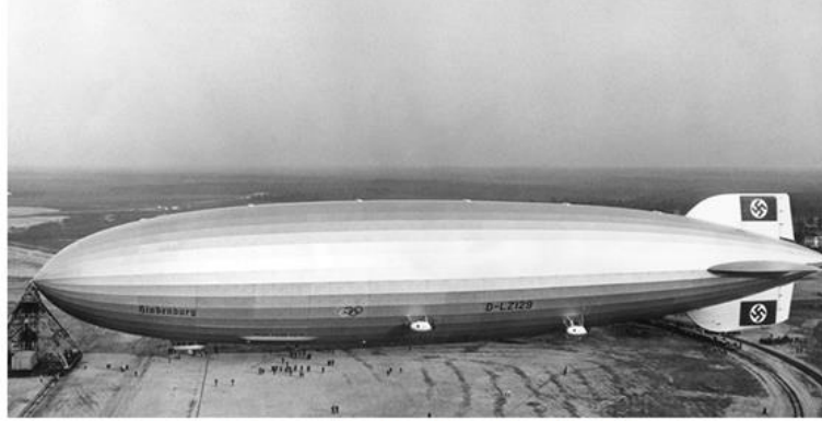
Zeppelin at the mast, illustrating the rail track for the tail
