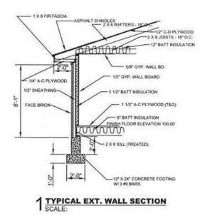
Volume of concrete (cf)= length (ft) x width (ft) x height (ft) Volume of concrete (cf)= 2'0'' x 2'0'' x 1'0'' = 4 cf x 14 footings = 56 cf Volume of concrete (cy)= 56 cf/ 27 cf per cy = 2.07 cy Add 5% for waste and round off Volume of concrete (cy)= 2.07 cy x 1.05 = 2.17 cy Use 3 cy
