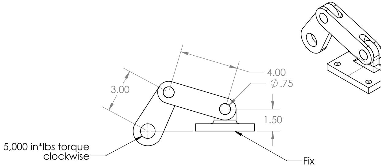
Design a slider crank mechanism using the layout shown. Your design should have a safe material of your choice.
