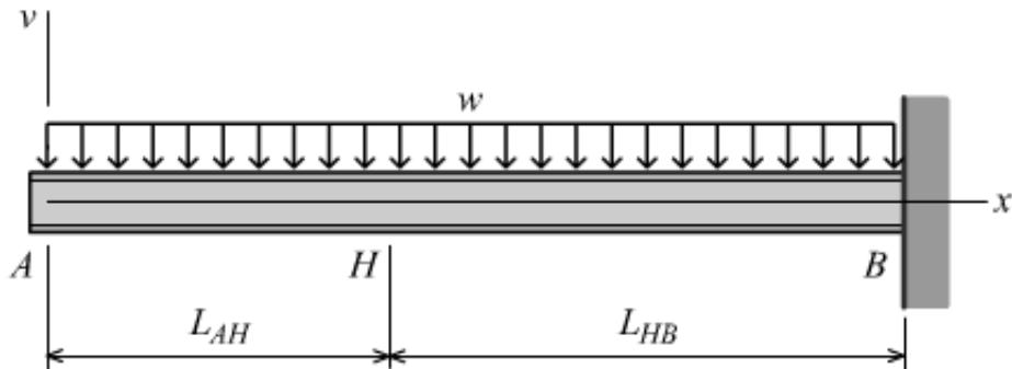
For Beam 3, determine the deflection at point H.
