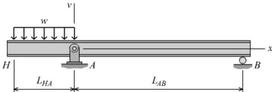
For Beam 4, determine the cantilever deflection of the beam at point H due to the uniformly distributed load 3.0 kips/ft between point A and point H. This is the deflection that would be calculated at point H assuming a fixed support at A.
