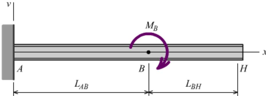
For Beam 1, determine the deflection and rotation angle at point  $B$ .
