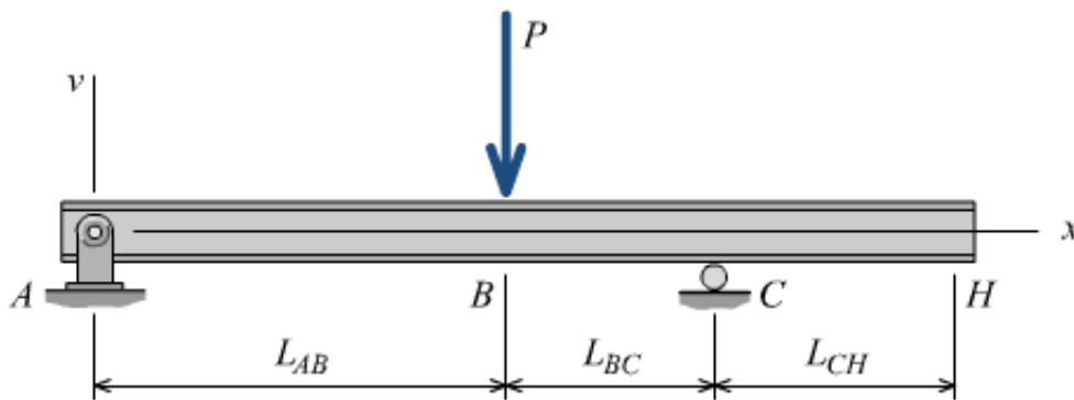
For Beam 2, determine the rotation angle at point C.
